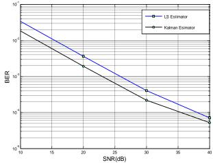
Figure 1. Performance of Least Square vs. Kalman channel estimators
