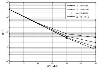
Figure 2. Doppler frequency effect on the least square estimator
