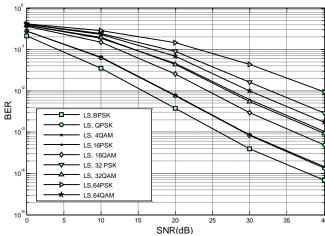
Figure 6. Performance of MPSK and MQAM modulation schemes, least square estimator
