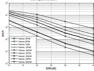
Figure 7. Performance of MPSK and MQAM modulation shcems ,Kalman estimator
