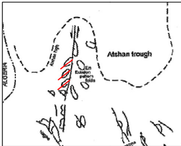
Figure-5.16: En echelon folding generated by left lateral transpressional strike slip faulting at the western part of Murzuq Basin striking NE-SW. After Echikh and Sola (2000).
