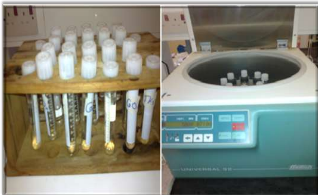
Figure (2.6): filtration and centrifugal of the samples for measuring EC and TDS.
