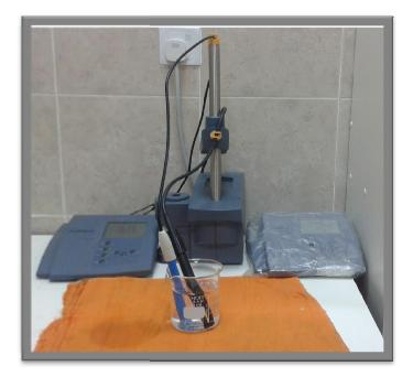
Figure (23). show Conductivity meter ( inolab cond 720) and pH meter (inoLab pH 720)
