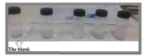
Figure (19). show the action between sample of water and reagent for detect the concentration of sulphate before set in Spectrophotometer
