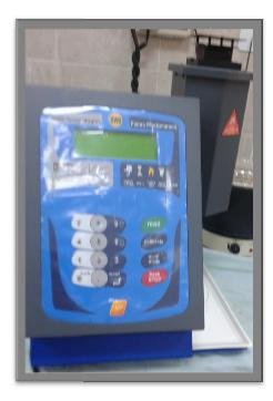
Figure (25). show flame photometer BWB technologies
