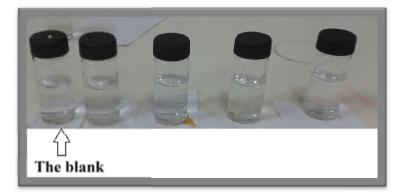
Figure (18). show the action between sample of water and reagent for detect the concentration of nitrite before set in Spectrophotometer
