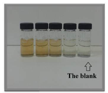
Figure (17). show the action between sample of water and reagent for detect the concentration of nitrate before set in Spectrophotometer
