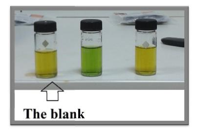
Figure (18). show the action between sample of water and reagent for detect the concentration of ammonia before set in Spectrophotometer
