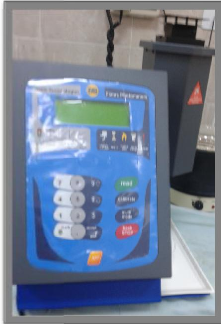
Figure (25). show flame photometer BWS technologies
