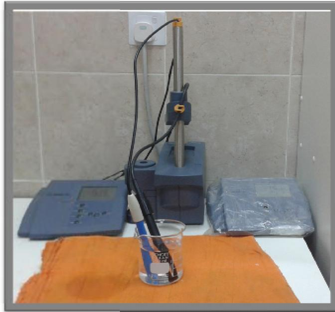
Figure (23). show Conductivity meter ( inoLab cond 720) and pH meter (inoLab pH 720)
