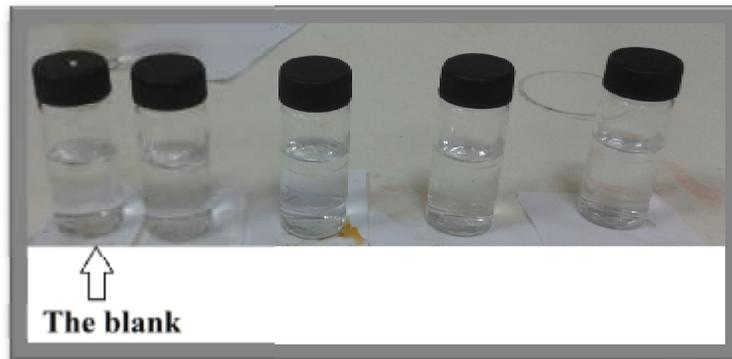
Figure (18). show the action between sample of water and reagent for detect the concentration of nitrite before set in Spectrophotometer
