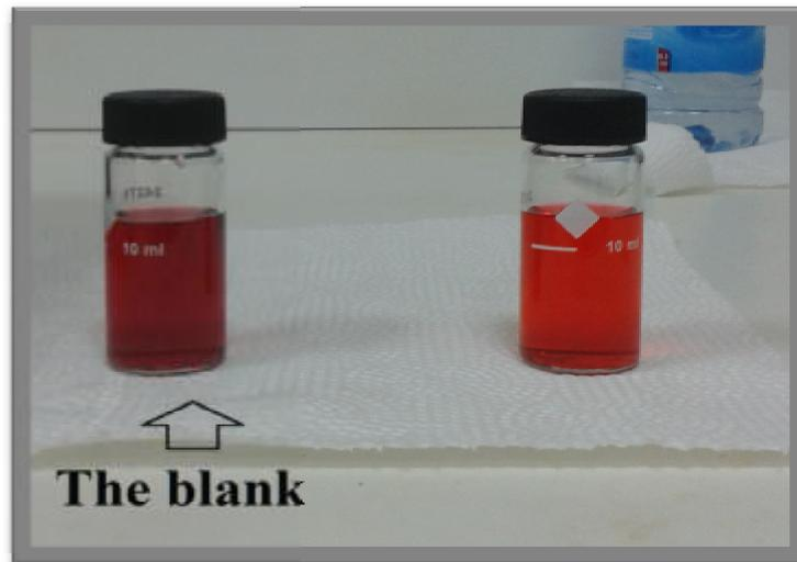
Figure (22). show the action between sample of water and reagent for detect the concentration of fluoride before set in Spectrophotometer
