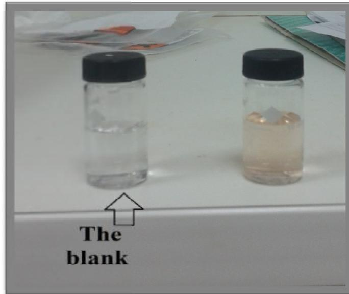
Figure (21). show the action between sample of water and reagent for detect the concentration of iron before set in Spectrophotometer
