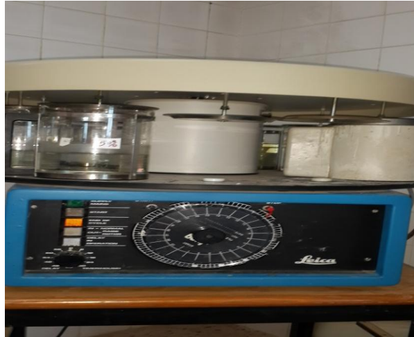
Figure2: histological processing machine for paraffin tissue processing steps.
