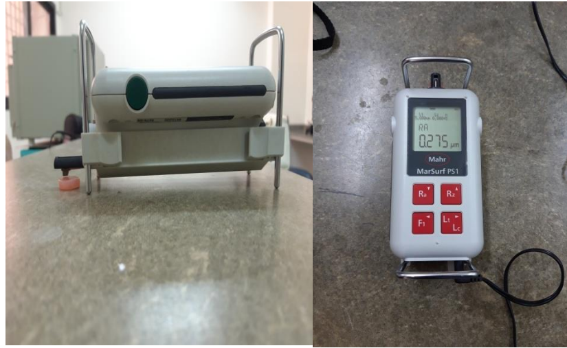
Figure 3.8: Surface roughness testing device(surface profilometer)
