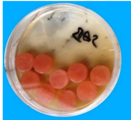
Figure 3.6: Tested samples in petri-dish incubated with microorganisms for colonization.
