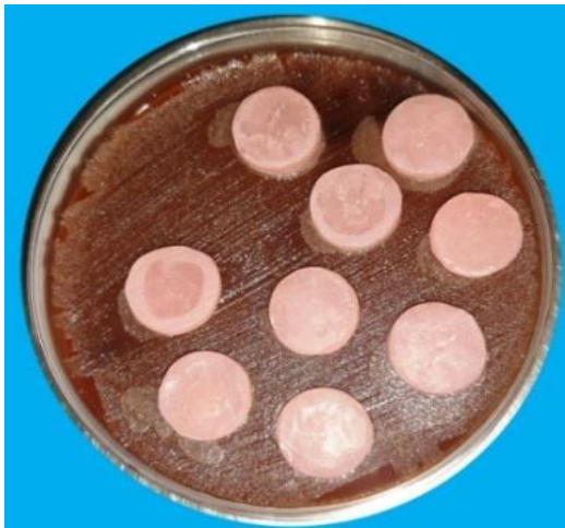
Figure 3.6: Tested samples in petri-dish incubated with microorganisms for colonization.
