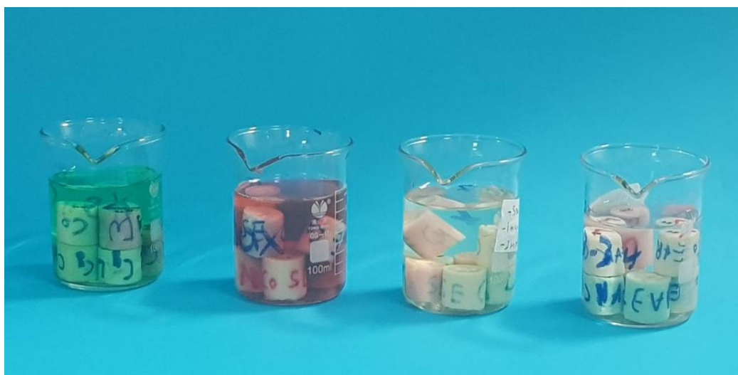
Figure 4.12: Four groups of specimens are soaking in four different disinfectant solutions.
