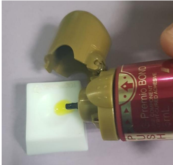
Figure 4.15: G-Premio Bond bonding agent in the dispensing well.
