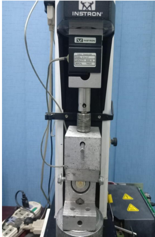
Figure 22: Composite bonded to dentin sample mounted on testing machine Instron machine
