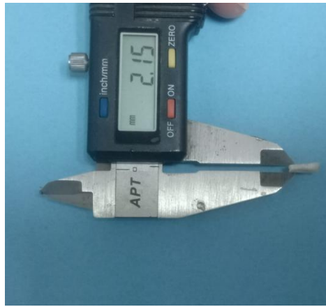
Figure 8: Sample thickness measured with APT
