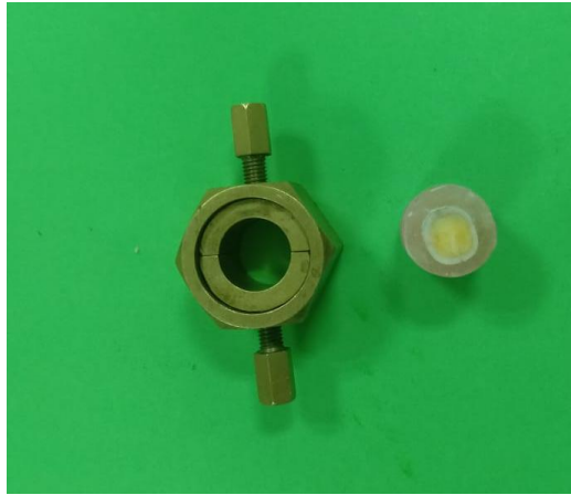
Figure 11: Sample of the dentin embedded in acrylic after removed from the mould.
