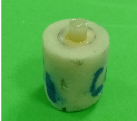
Figure 21: The prepared Sample after removal of Teflon mould.
