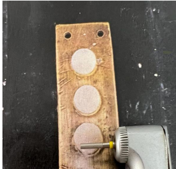
Figure 4.6: photographic image of finishing and polishing procedures by diamond bur
