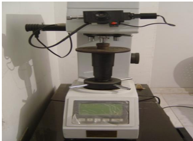
Figure 4.10: Photographic image of Digital Display Vickers Micro-Hardness Tester used for hardness measurement.
