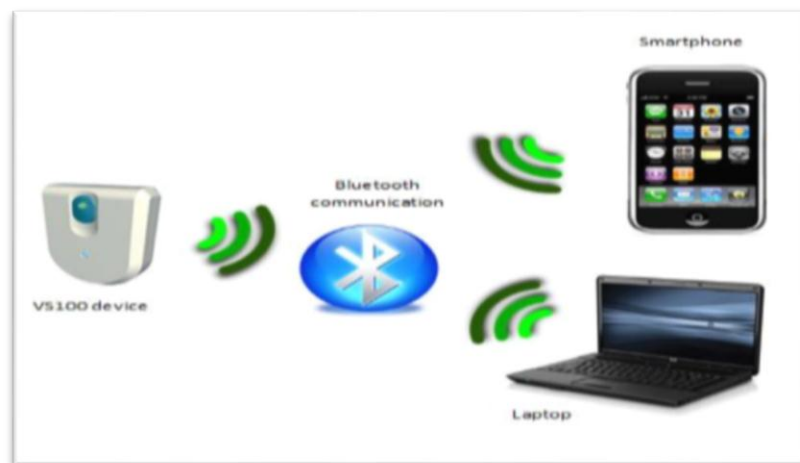
Figure (2.12): System overview of Vitalsens Vs100.[11]
