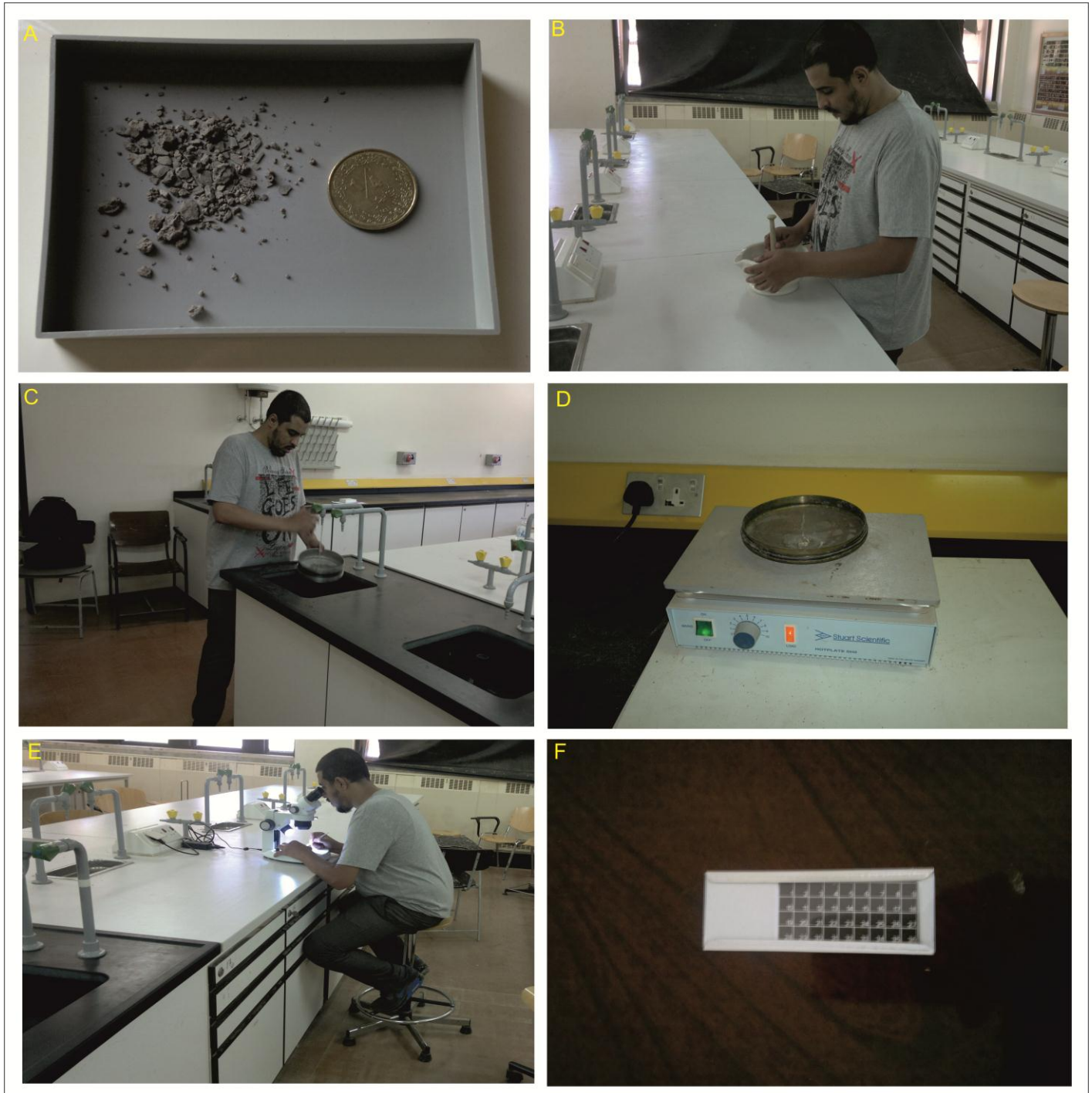
Fig. 1.8 A) the received quantity of ditch cutting sample; B) crushing the sample; C) washing the sample through 63 \mu\text{m} sieve; D) drying the sample on a hotplate; E) examining the sample residue under a stereomicroscope and picking up the foraminifers; F) mounting the foraminifers in a labeled micropaleontologic slides.
