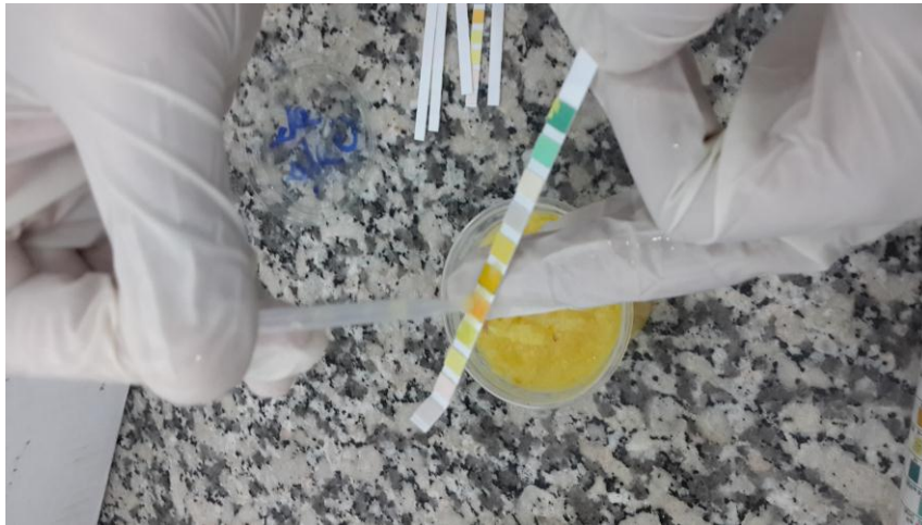
( Fig. 4.51 ) The measurement of pH peel juice , pH sac juice and pH whole fruit juice .
