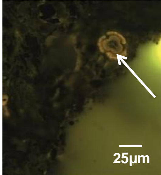
Fig. 2.12: Photomicrograph showing resinite (white arrow, sample Q14).
