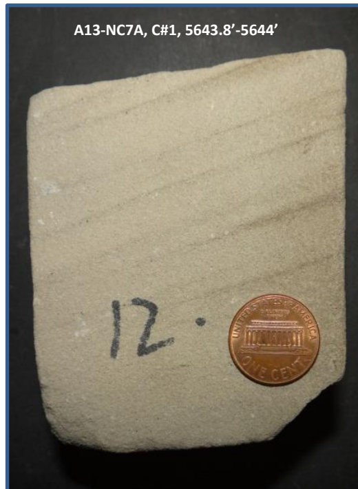
Figure 26. Slabbed core sample of lithofacies (7) in Tahara Formation, in well (A13-NC7), concession NC7A, Ghadames Basin showing, planar laminated sandstone with angular basal contact and current direction from right to left.
