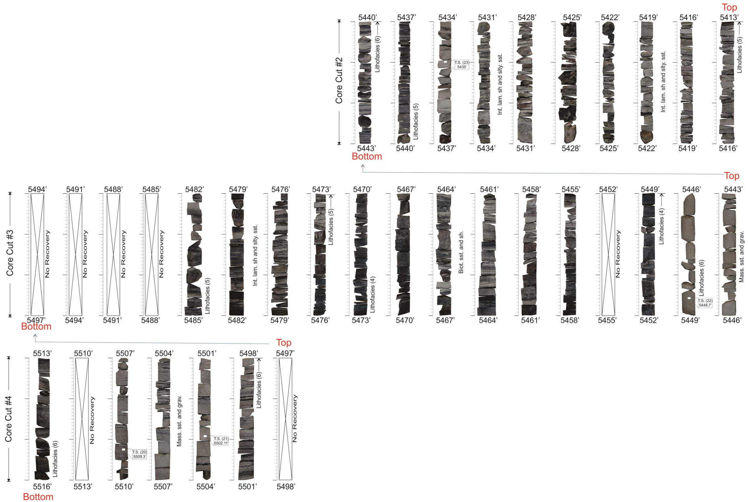
App.I.13. Photograph of cores #2 (5413'-5443'), #3 (5443'-5497'), #4 (5497'-5516'), of Tahara Formation in well F1-26, concession NC7A, Ghadames Basin. (Detailed description of lithofacies are included in App.I.14 and App.I.15).
