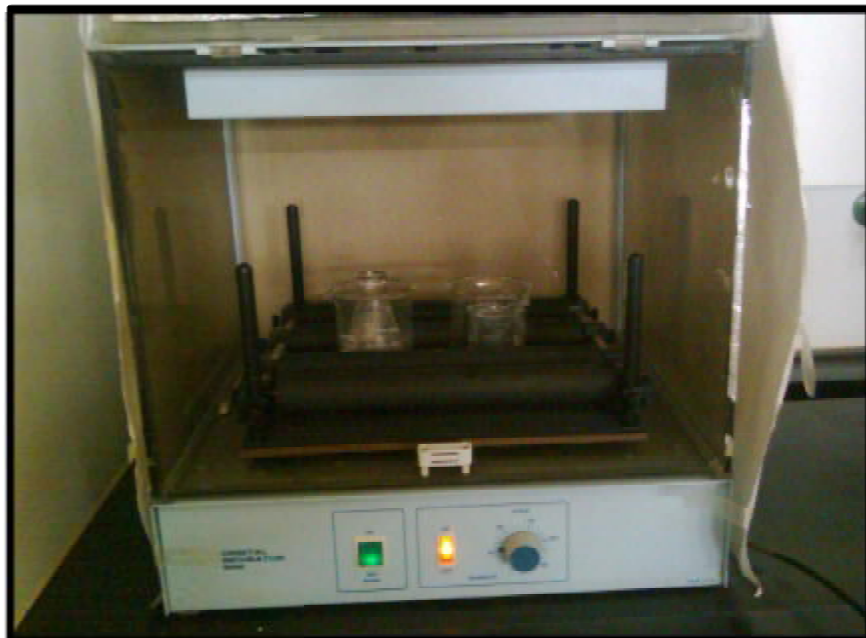
Figure (6): Shows an incubator with a water bath trembling used for oocysts sporulation .
