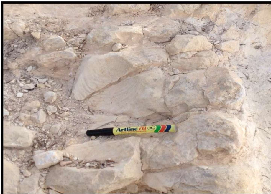
Fig. (2.7) Marly limestone in Al Majahir Formation showing the internal mold of Inoceramus shell.
