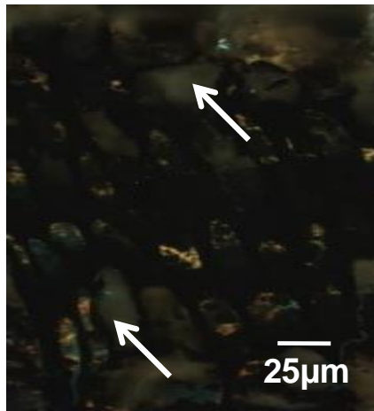
Fig. 2.2: Photomicrograph showing densinite (white arrows, sample D10).
