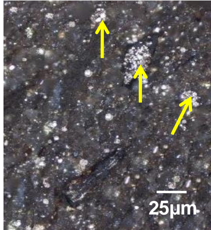
Fig. 2.15: Photomicrograph showing inertodetrinite (yellow arrows, sample D4).
