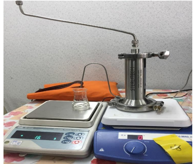
Figure 3. The dead-end permeation cell.
