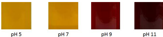
Fig.10. Zoomed photographs taken with digital camera to investigate colour changes of curcumin solution at different pH values.
