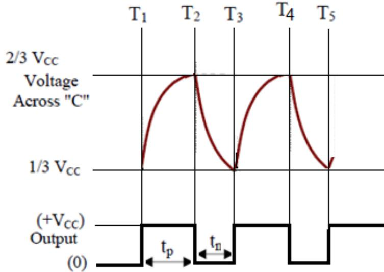
Figure. 2. The output signal for the Astable 555 timer
