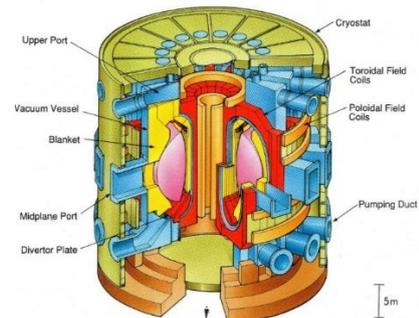
Fig. 2. International thermonuclear Experimental Reactor with Divertor Facilities, (courtesy of ITER Group).
