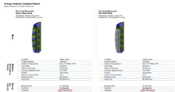
Fig. 2.16: Building energy analysis result (Vasari software)
