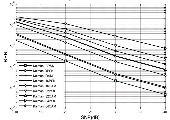
Figure 7. Performance of MPSK and MQAM modulation schemes, Kalman estimator
