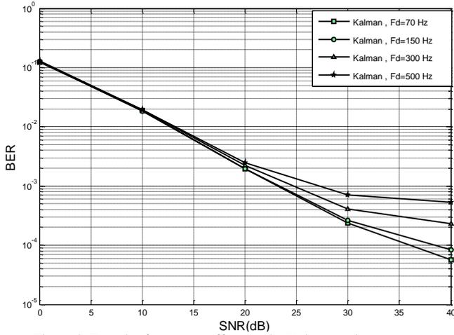
Figure 3. Doppler frequency effect on the Kalman estimator
