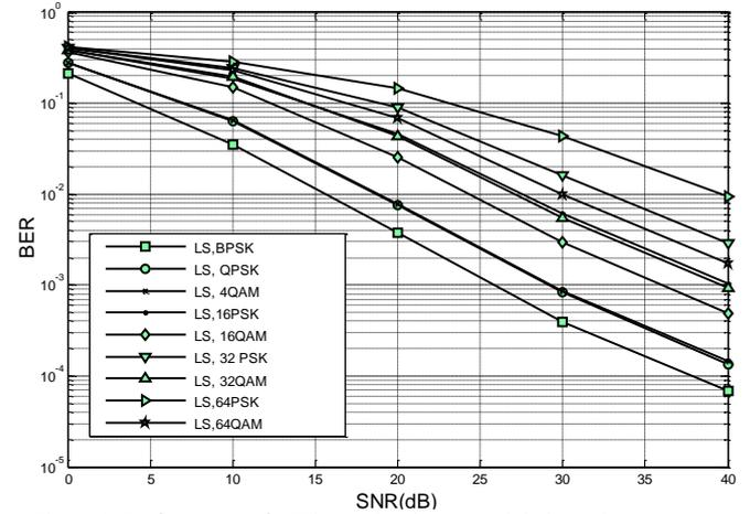
Figure 6. Performance of MPSK and MQAM modulation schemes, least square estimator
