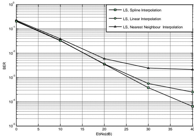
Figure 4. Interpolation methods using Least Square estimator
