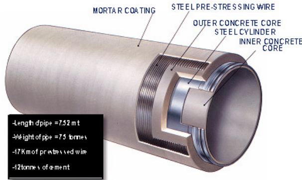
Figure 3: PCCP Material Components
