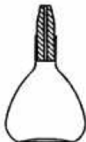
Figure 2.2: The pycnometer using to determination of density
