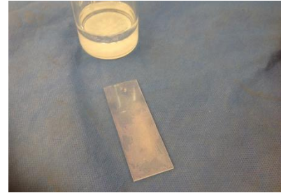
Fig. 2. Photograph shows of ZnS thin film formed at the water/toluene at 60°C.
