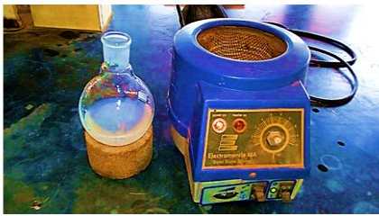
Fig. 1. photograph shows the preparation of ZnS colloid in the presence of a capping agent.
