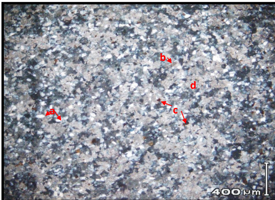
Figure 65. Thin section photomicrograph (12) of Quartzarenite in basinal silt/shale in Memouniat Formation, showing (a) quartz, (b) feldspar, (c) clay clasts and (d), pervasive calcite cement. Core # 15 at 6302.3ft., well D1-23 (XPL).
