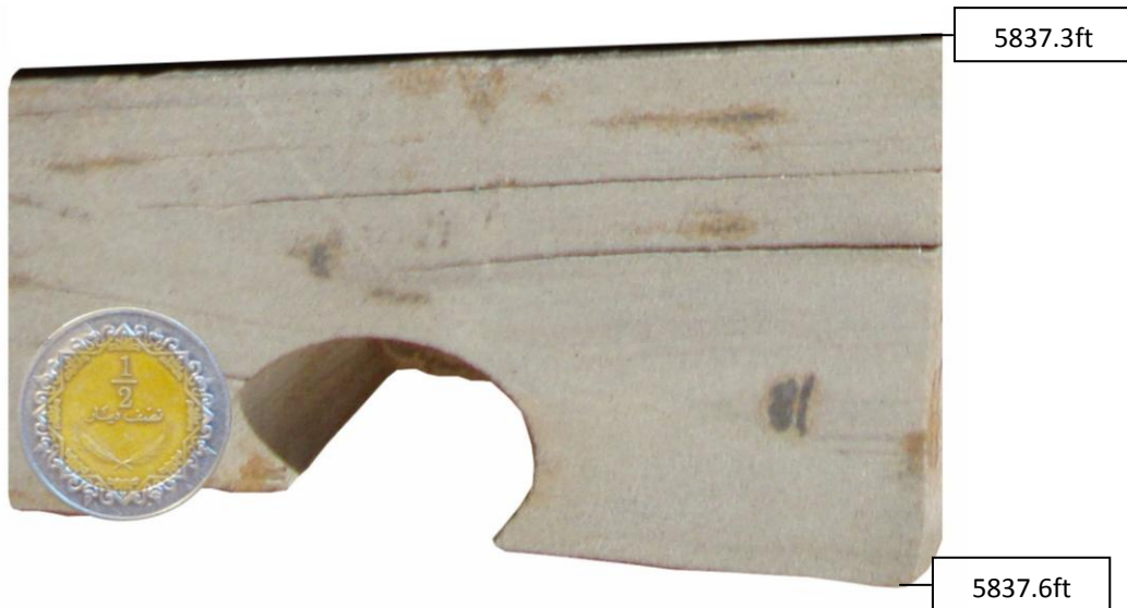
Figure 31. Truncated surface primary sedimentary structures in proximal sands predominated sector, core #12 (5828.8-5843.8ft) in well A1-NC1.
