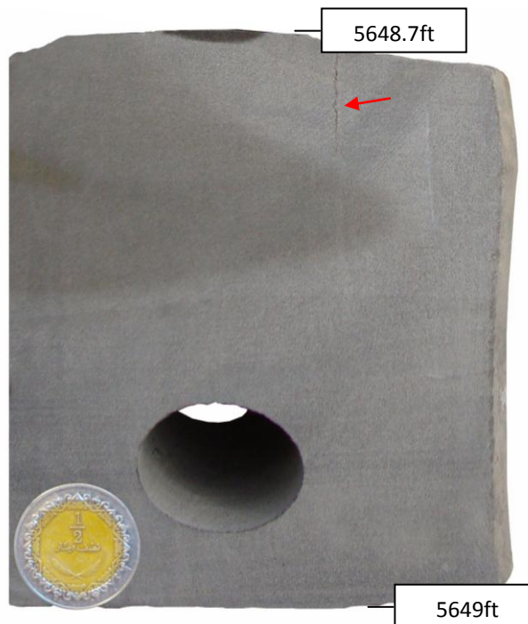
Figure 38. Micro fracture structures (indicated by arrows) in proximal sand predominated sector, core #11 (5641-5657ft) in well A1-NC1.
