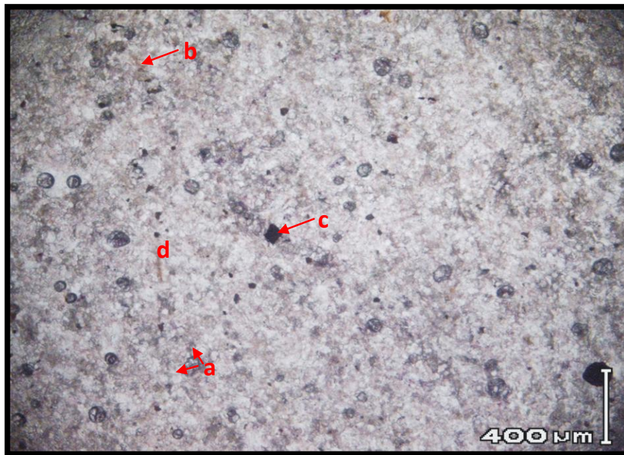
Figure 62. Thin section photomicrograph (11) of Quartzarenite in basinal silt/shale in Memouniat Formation, showing (a) quartz, (b) feldspar, (c) clay clasts and (d) pervasive calcite cement. Core # 15 at 6301.4ft., well D1-23 (PPL).
