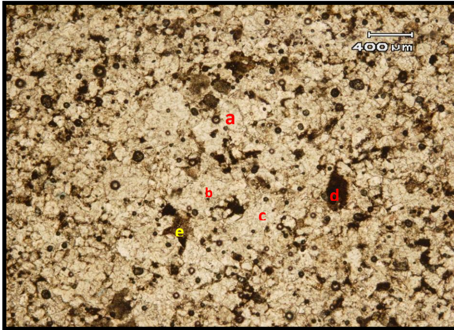
Figure 49. Thin section photomicrograph (5) of Sublitharenite in channel fill sands in Memouniat Formation, showing (a) quartz, (b) feldspar, (c) polycrystalline quartz, (d) clay clasts and (e) calcite cement. Core # 3 at 6166.69ft., well GG1-66 NC8A (PPL).
