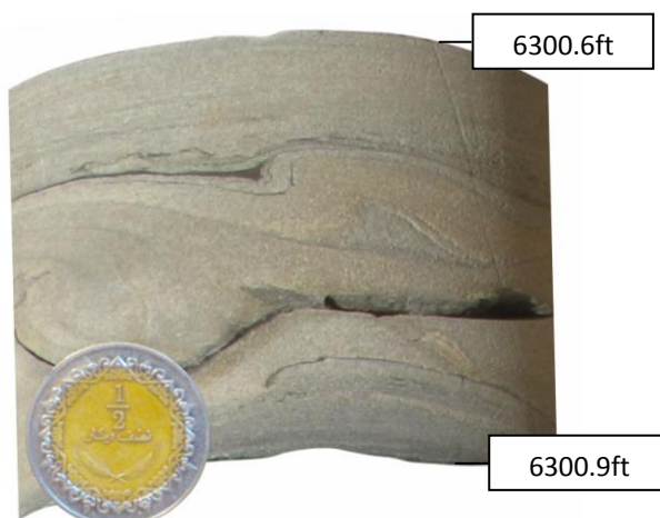
Figure 36. Slump like structure in basinal silt/shale predominated sector, core #15 (6256-6311.6ft) in well D1-23.
