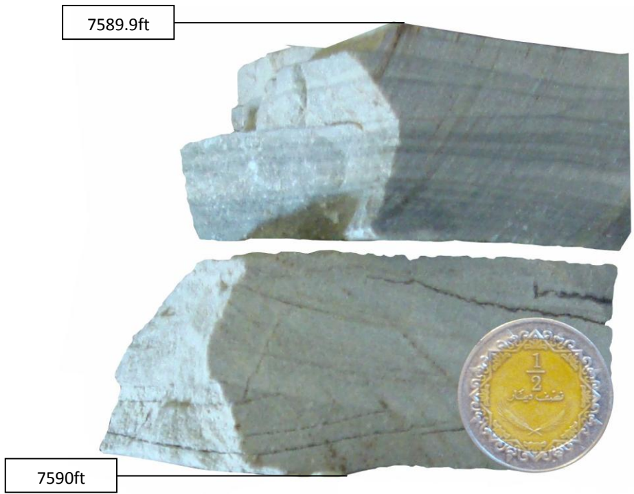
Figure 23. Trough x-lamination in channel fill sands facies predominated sector, core #11 (7598-7570ft) in well F1-66.
