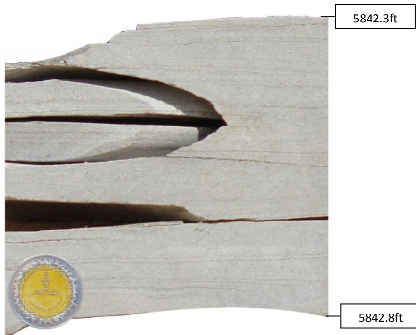
Figure 30. Horizontal and wavy lamination primary sedimentary structures in proximal sands predominated sector, core #12 (5828.8-5843.8ft) in well A1-NC1.
