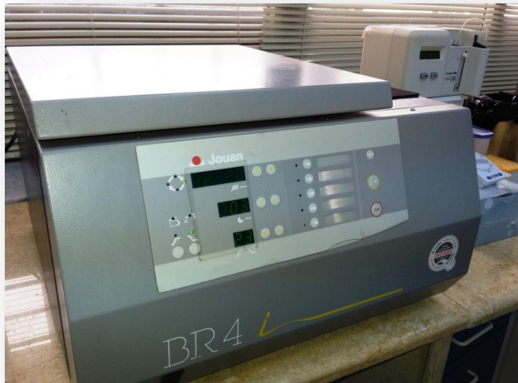
Figure 6: Centrifuging machine for blood and saliva samples.
