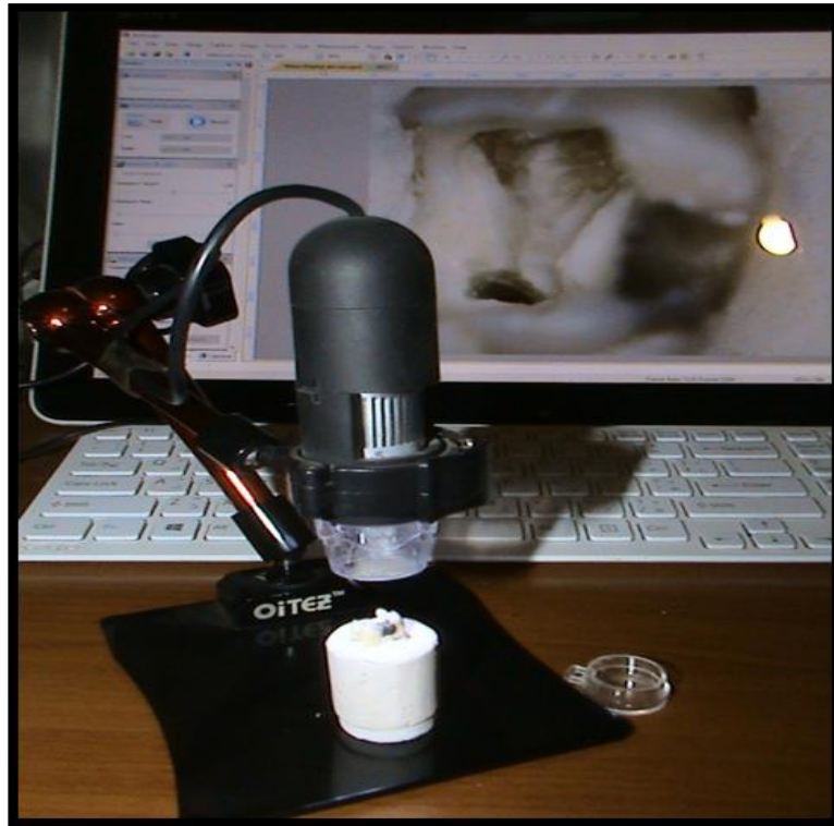
Figure 18: Oitez usb digital camera (20x-800x). linked to computer and used during procedure for photographing the samples.
