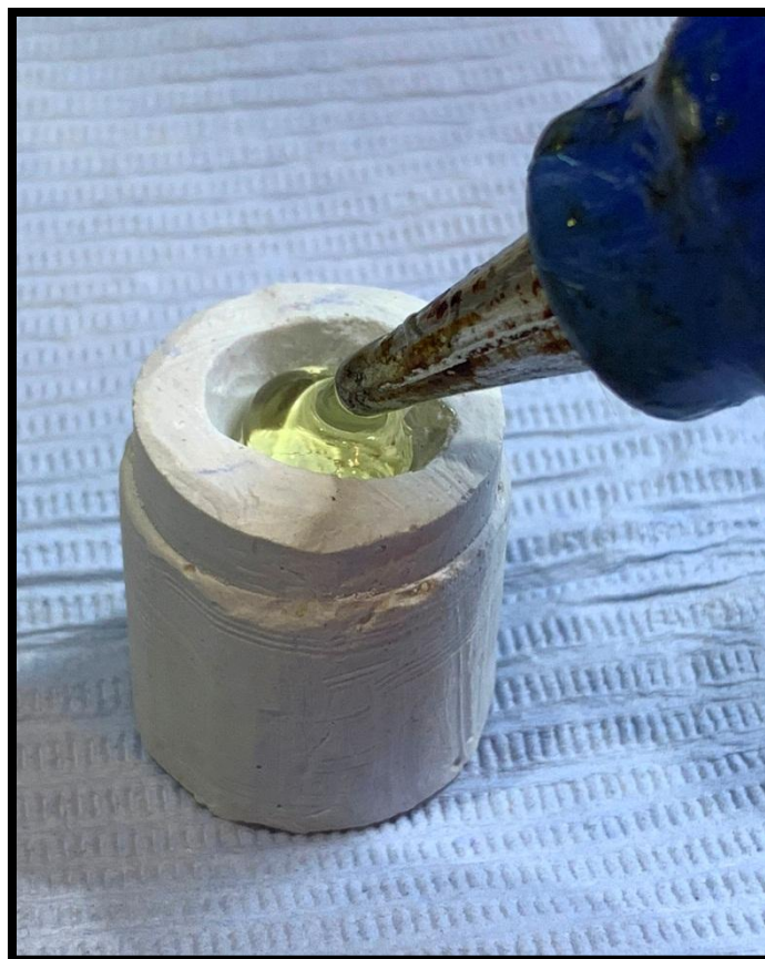
Figure 2: A glue gun used for injection of hot melt translucent stick in the hole of the custom made plaster block.
