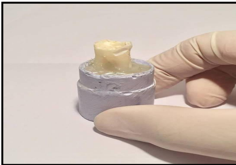
Figure 3: Sample was mounted into the glue hole of the plaster block to facilitate the handling during access cavity preparation.
