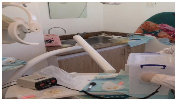
Figure 4.3: Teeth grinding done by using a cylindrical alpine tooth grinding stone fitted to a straight hand piece (micro-motor unit Kavo, EWL K-11) inside a transparent plastic box.
