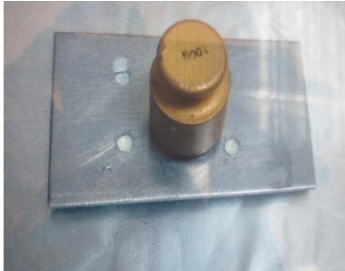
Figure 3.4: put of 100g load over top glass slap until complete setting of material
