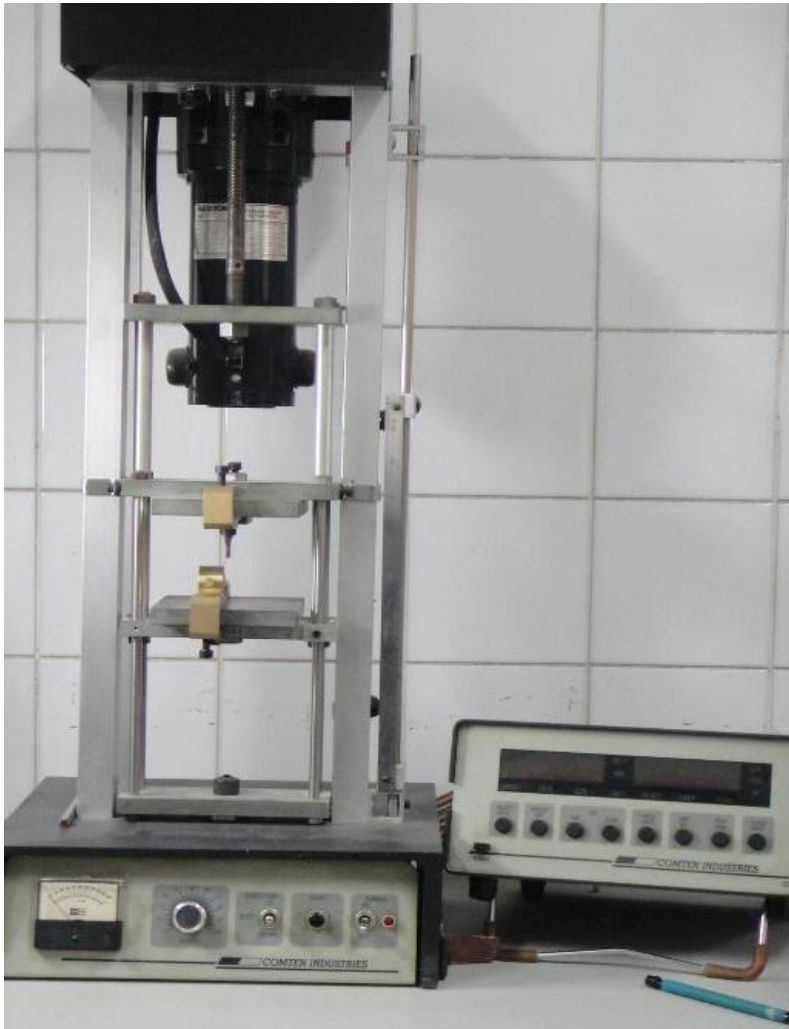
Figure 16: Universal testing machine Comten industries, Inc. St .Petersburg, Florida, USA, Model No .942D10-20.
