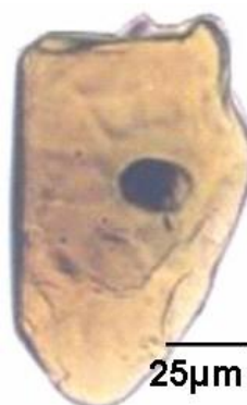
Fig. 2.33: Photomicrograph showing subrounded brown biotite grain (sample 4c).
