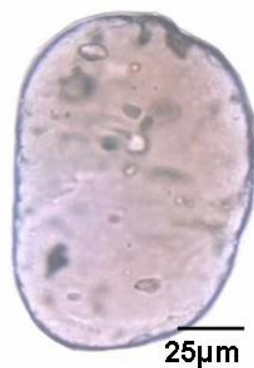
Fig. 2.24: Photomicrograph of well rounded pink tourmaline grain (sample 3c).
