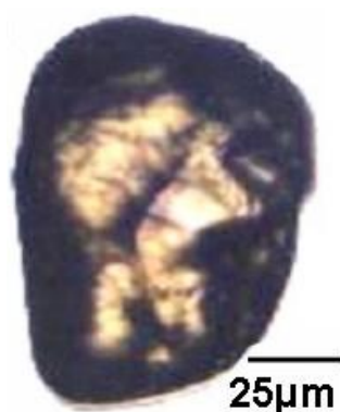
Fig. 2.35: Photomicrograph of rounded monazite grain (sample 5e).
