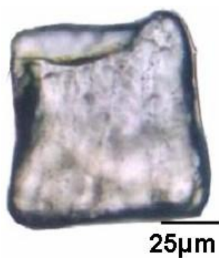
Fig. 2.25: Photomicrograph of cubic garnet grain (sample 2c).
