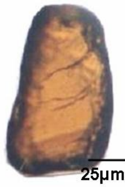
Fig. 2.30: Photomicrograph showing reddish brown elongated rounded rutile grain (sample 2b).
