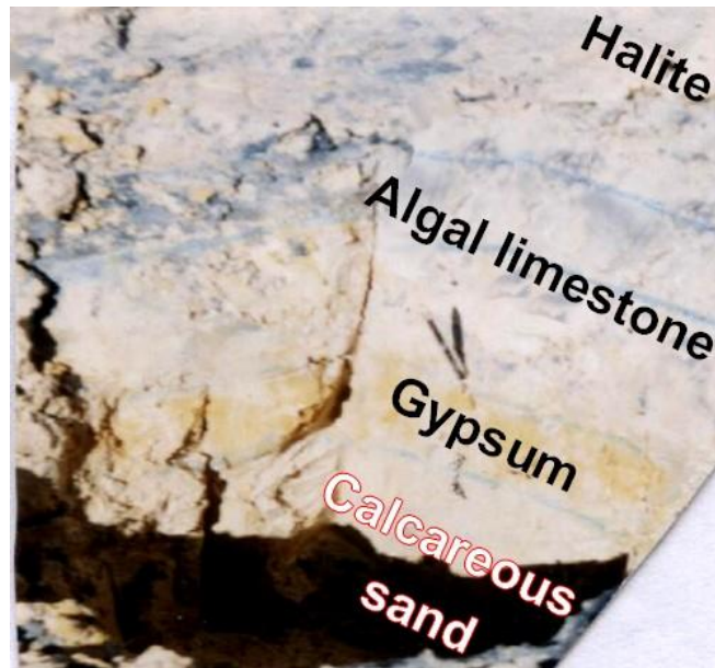
Fig. 2.7: Lithology of sabkha profile at the station no. 3 (Abu Kammash).
