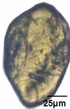
Fig. 2.29: Photomicrograph of subrounded pistachite grain (sample 3c).
