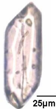
Fig. 2.27: Photomicrograph of prismatic bipyramidal zircon grain (sample 3c).
