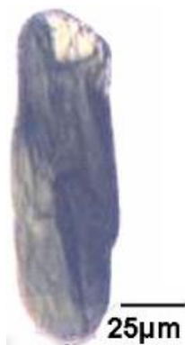
Fig. 2.36: Photomicrograph of prismatic augite grain (sample 3c).
