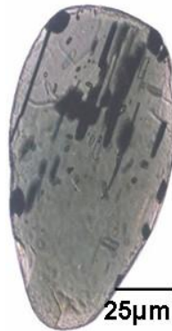
Fig. 2.32: Photomicrograph showing subrounded bluish green hornblende grain (sample 4c).
