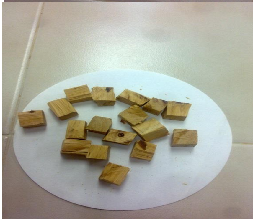
(Figure 3.6) Prepared wood blocks with diameter (2 \times 1.5 \times 1.5 \text{ cm}^3) 20 mm x 15 mm x 1.5 mm , in the longitudinal directions (L) ,radial (R) and tangential (T) .
