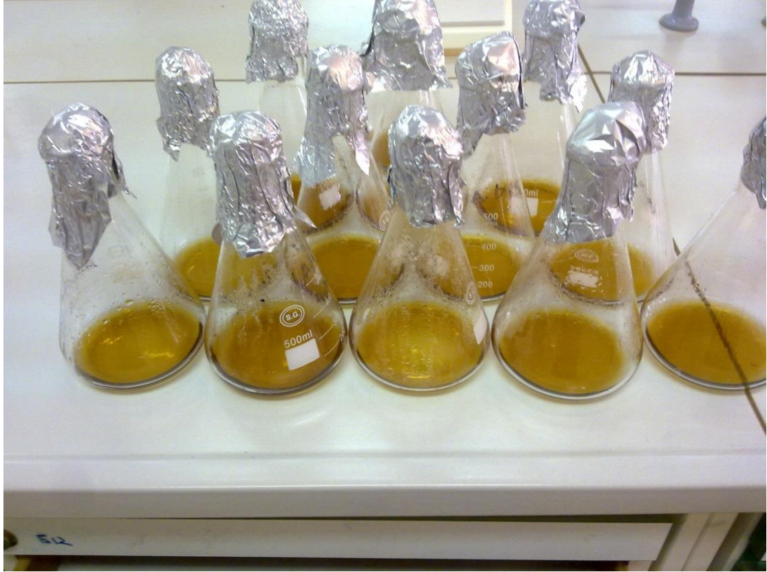
(Figure 3.7) Conical flasks contain a sterilized PDA before inoculation of isolated wood – decay fungi .
