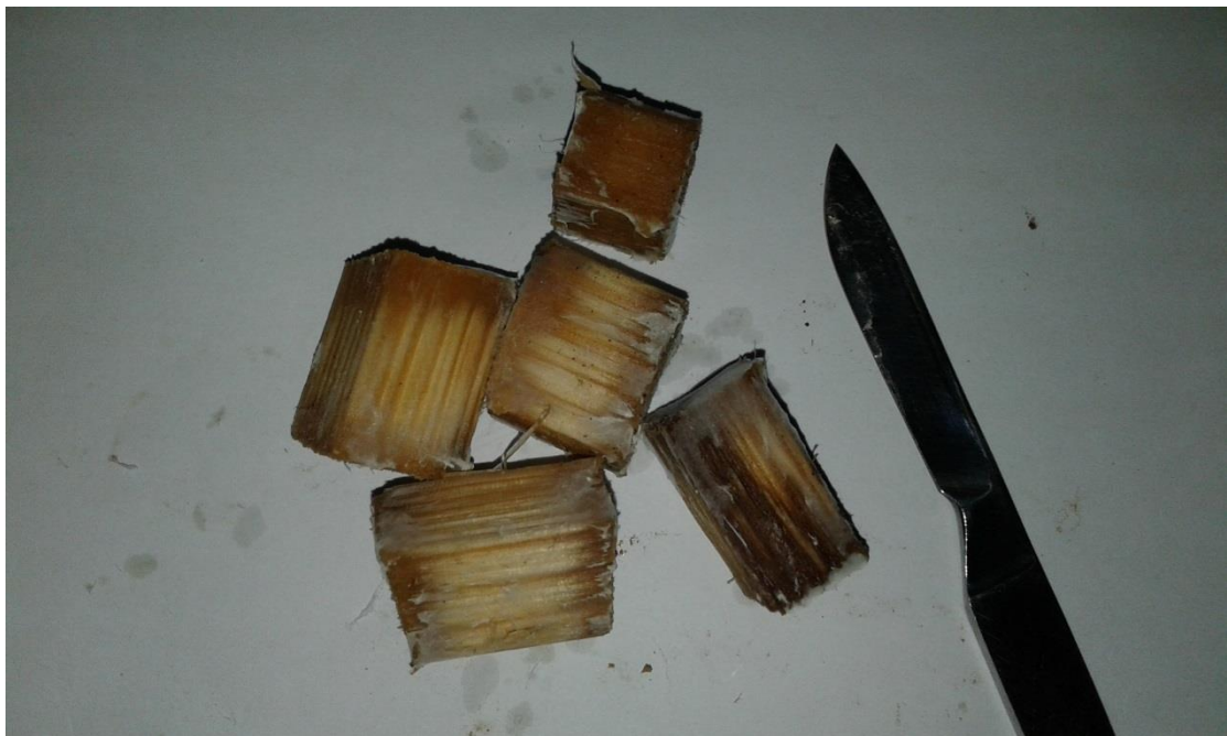
(Figure 3.9) The treated blocks were removed and their surfaces were scraped free of mycelium and nutrient medium by using lancet .
