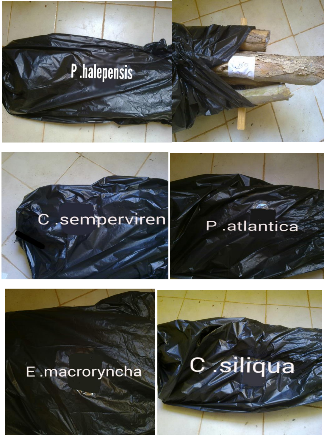
(Figure 3.4) The samples were kept in well-sealed black bags at room temperature (20-30°C) and stored in the lab for 8 weeks , to reduce the moisture content after weighted and organized in groups .
